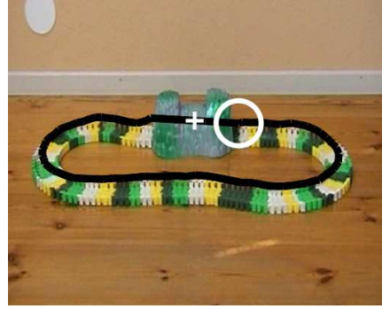
FIGURE 2: The track with the car in the tunnel. The system is waiting for the car to reappear at the end of the tunnel to the right. The previously predicted path of the car (black line), the currently predicted location (white cross) and the attended location (white circle).
